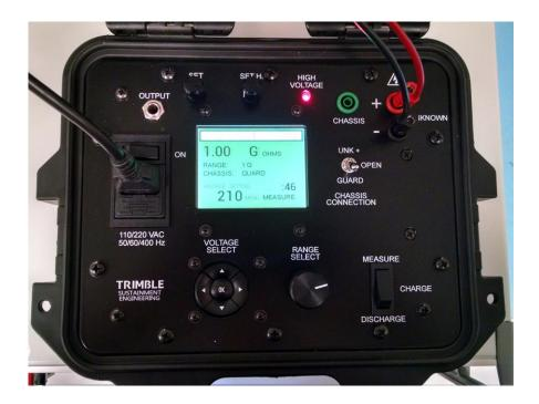
The output voltage of the EM1001A can be set in 1VDC steps from 10 to 1100 VDC with an accuracy across the entire range of  $\pm$  1% of setting, allowing for non-standard voltage configurations to cover many applications.
