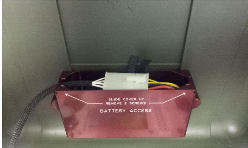
**FIGURE 6. BATTERY PROPERLY INSTALLED**
