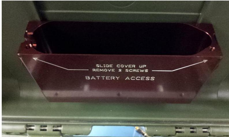
FIGURE 4. BATTERY BOX COVER REMOVED
