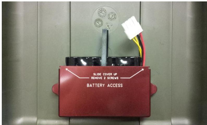
FIGURE 5. BATTERY PARTIALLY INSTALLED
